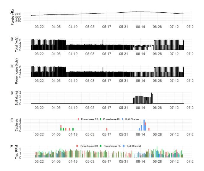
Figure 7. Forebay elevation (panel A), total outflow (panel B), powerhouse flow (panel C), spill (panel D), daily Chinook salmon catch (panel E), and trapping effort in mean revolutions per minute (panel F) below Lookout Point Dam. Trapping effort is calculated as trap revolutions divided by the number of minutes elapsed since the trap was last checked. RL and RR stand for river left and river right, respectively.
