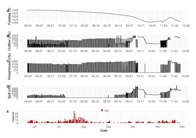
Figure 17. Forebay elevation (panel A), total outflow (panel B), powerhouse flow (panel C), and spill (panel D) at Detroit Dam, along with the number of Chinook salmon captured below Big Cliff Dam (panel E), 2021.
