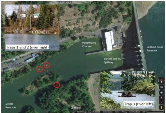
Figure A- 3. Rotary screw trap locations below Lookout Point Dam, 2021. Red circles indicate trap fishing location (two 2.4 m traps in the powerhouse channel (river right) and a 2.4 m trap in the surface and RO spillway channel (river left).
