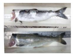
Figure C-12. Body only (BO – mechanical damage)
