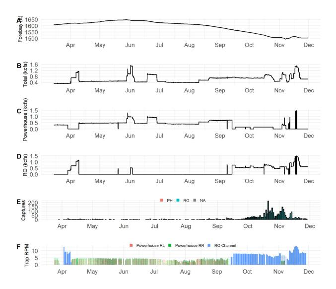
Figure 10. Forebay elevation (panel A), total outflow (panel B), powerhouse flow (panel C), spill (panel D), captured Chinook salmon (panel E), and trapping effort (panel F) below Cougar Dam, 2021. Trapping effort is calculated as trap revolutions divided by the number of minutes elapsed since the trap was last checked. RL and RR stand for river left and river right, respectively.
