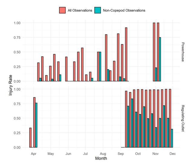
Figure 11. Weekly injury rate observed in juvenile Chinook captured below Cougar Dam in the powerhouse channel (top panel) and the regulating outlet (bottom panel). Red bars depict the injury rate with the presence of copepods counting as an injury. Blue bars depict the injury rate not including copepods.
