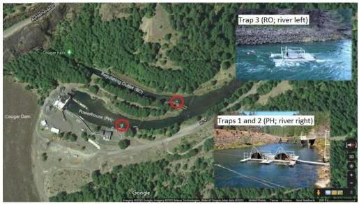
Figure A- 2. Rotary screw trap locations below Cougar Dam, 2021. Red circles indicate trap fishing location (two 2.4 m traps in the powerhouse/tailrace channel (PH; river right) and a 1.5 m trap in the regulating outlet (RO; river left).
